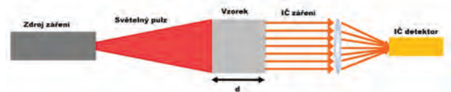
Obr. 6: Schéma LFA metody [8]
